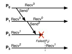
Fig. 6: Using the receive function modeled after the  $FT\_Send\_right$  function (seen in Figure 5), the application hangs when  $P_2$  fails after receiving the message from  $P_1$ , but before sending it to  $P_3$ .
