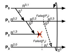
Fig. 7: Using the receive function from Figure 9,  $P_1$  notices the failure of  $P_2$  and resends the message to  $P_3$ .
