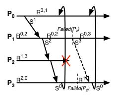
Fig. 8: Using the receive function from Figure 9,  $P_3$  receives the same message twice (once from  $P_2$  before it fails, and from  $P_1$  as a resent message). This causes the iteration to complete twice, when there is no control for duplicate messages.
