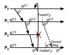
Fig. 10: By using the iteration marker to discard duplicate messages during the receive (seen in Figure 9) the ring iteration is able to complete without duplicating messages.
