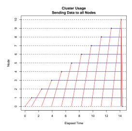
Figure 1: Visualization of timing information for cluster usage for component test 1 with the **snow** package using MPI. Green rectangles representing active computation (in this case very small), blue horizontal lines representing a worker waiting to return a result, and red lines representing master-slave communications.
